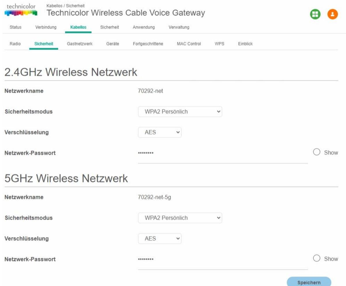
The screenshot shows the web interface for a Technicolor Wireless Cable Voice Gateway. The navigation menu includes 'Status', 'Verbindung', 'Kabellos', 'Sicherheit', 'Anwendung', and 'Verwaltung'. Under 'Kabellos', there are sub-menus for 'Radio', 'Sicherheit', 'Gastnetzwerk', 'Geräte', 'Fortgeschrittene', 'MAC Control', 'WPS', and 'Einblick'. The 'Sicherheit' sub-menu is active, showing settings for two wireless networks: 2.4GHz and 5GHz.
