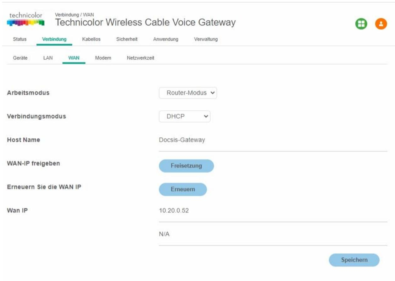
The screenshot shows the WAN configuration interface for a Technicolor Wireless Cable Voice Gateway. The page title is "Technicolor Wireless Cable Voice Gateway" and the current section is "Verbindung / WAN". The "WAN" tab is selected in the navigation menu. The configuration options are as follows:
